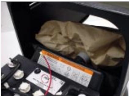
The Vac-Trac™ Dust Control System collects pad dust and deposits it in a 115.5 in. 3 filter bag at the front of the machine.
